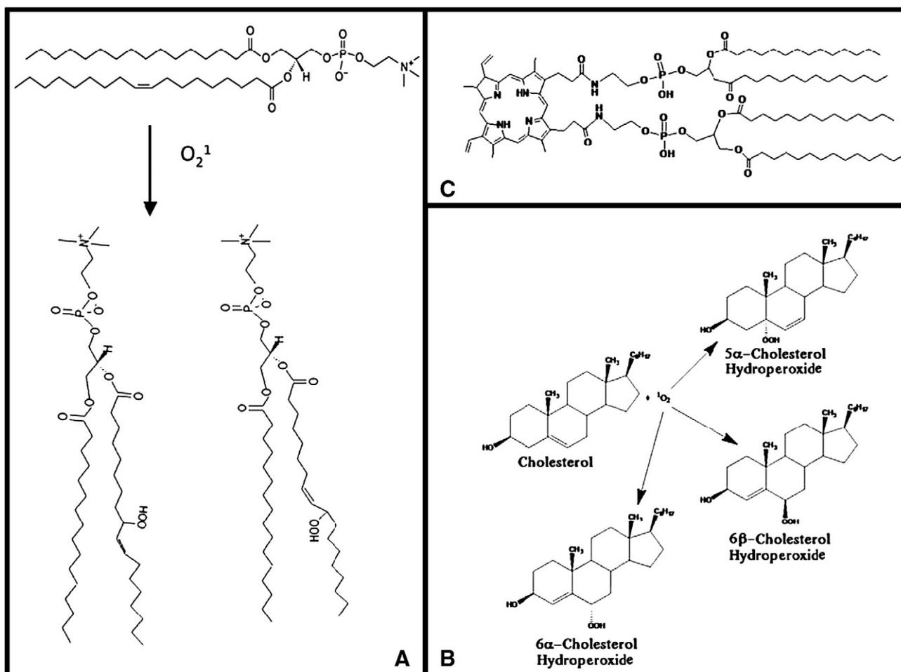
Fig. 1. Molecular structure of the hydroperoxides formed during the photo-oxidation reaction of POPC (A) and cholesterol (B) via singlet oxygen  $O_2^1$ . Chemical structure of the photosensitizer PE-porph, which consists of a porphyrin attached to the headgroups of two molecules of phosphatidylethanolamine (C).
